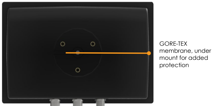
Figure 3: CCpilot V700 rear side view
